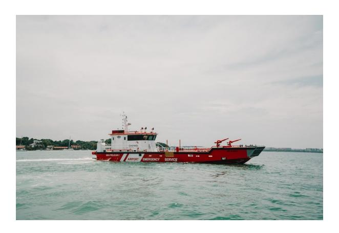
The newly commissioned Landing Craft (above) replaced the previous hovercraft with enhanced capabilities while maintaining the same core functions – firefighting and casualty management. With a capacity of 50 passengers, and the ability to reach speeds of up to 40 knots, this vessel is versatile for sea rescue operations.
